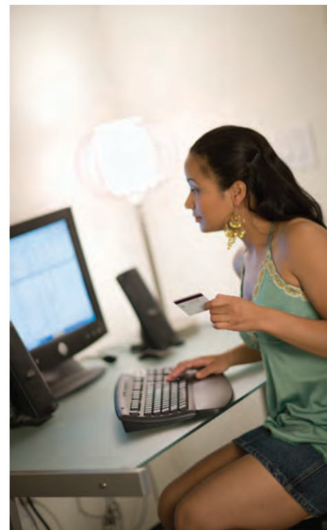
Figure 5.20 This keyboard has an ergonomically designed wrist support. It helps prevent repetitive strain injury.
