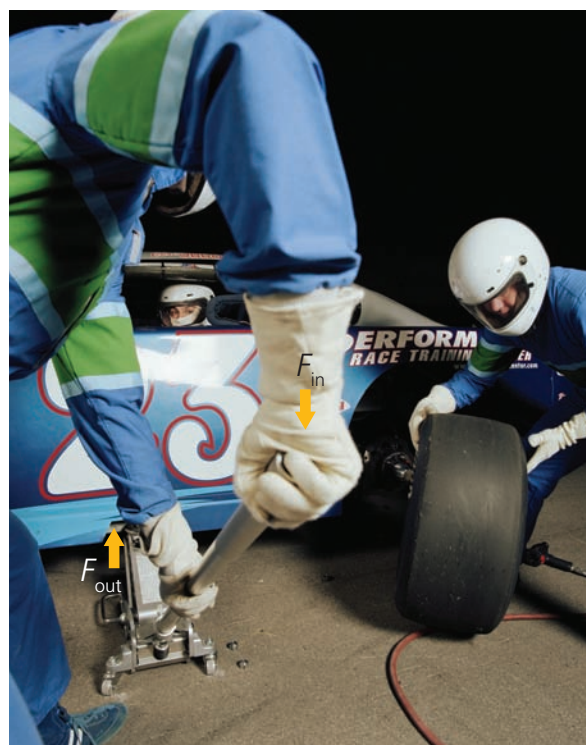
Figure 4.24 The input force, F_{\text{in}} , and output force, F_{\text{out}} , using a car jack
