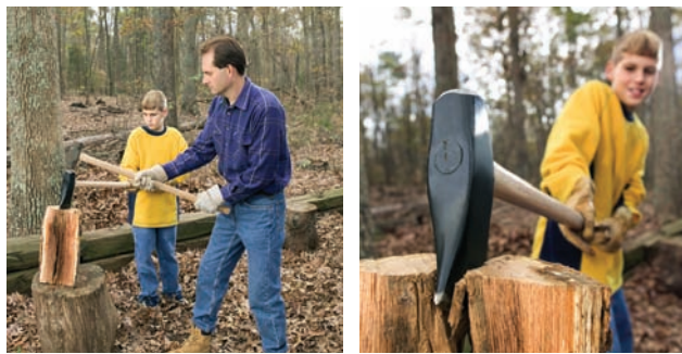
Figure 5.26 A wedge is an inclined plane that moves through the object.
