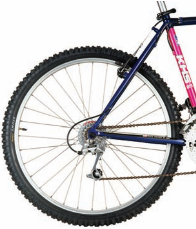
Figure 5.21 Since the input force is applied closer to the axle than the output force on the rim, this bike wheel has an IMA less than 1.
