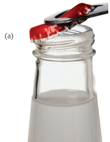
Figure 5.8 A bottle opener (a) is an example of a second-class lever, which has the output force between the fulcrum and the input force (b).
