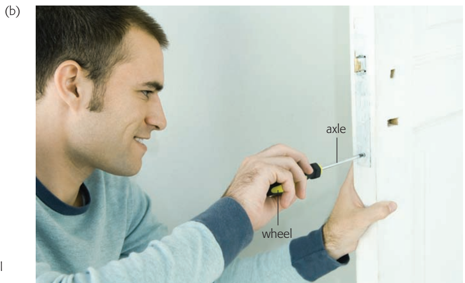
Figure 5.20 (a) A wheel and axle. (b) A screwdriver is an example of a wheel and axle.
