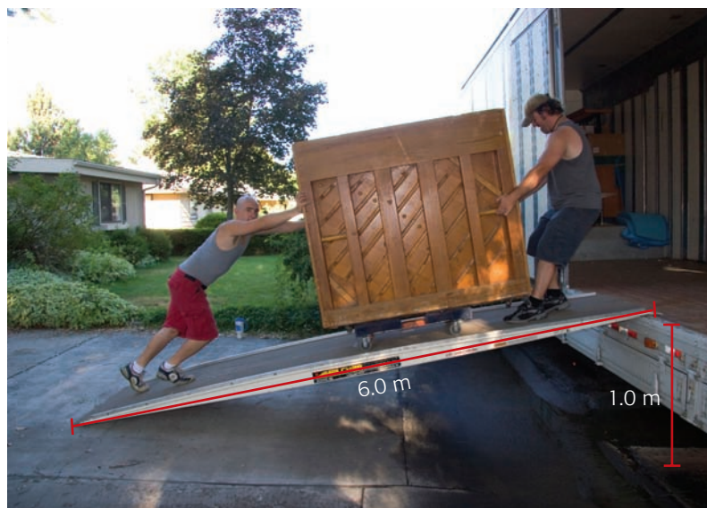
Figure 5.24 An inclined plane allows you to use less force over a greater distance.
