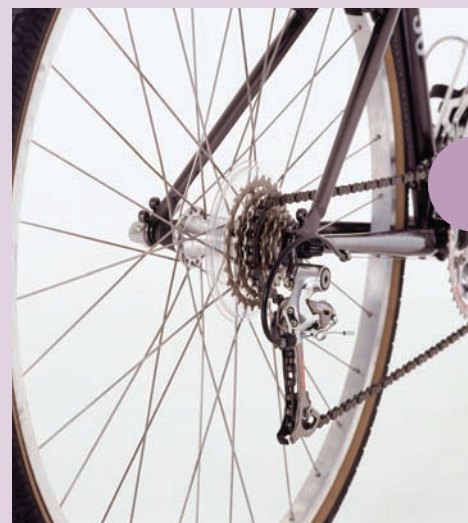
Figure 5.3 The mechanical advantage can be changed by moving the chain to different sprockets.
