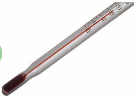
Figure 7.13 When the temperature drops, the particles in the tube move closer together and the level of liquid falls.
