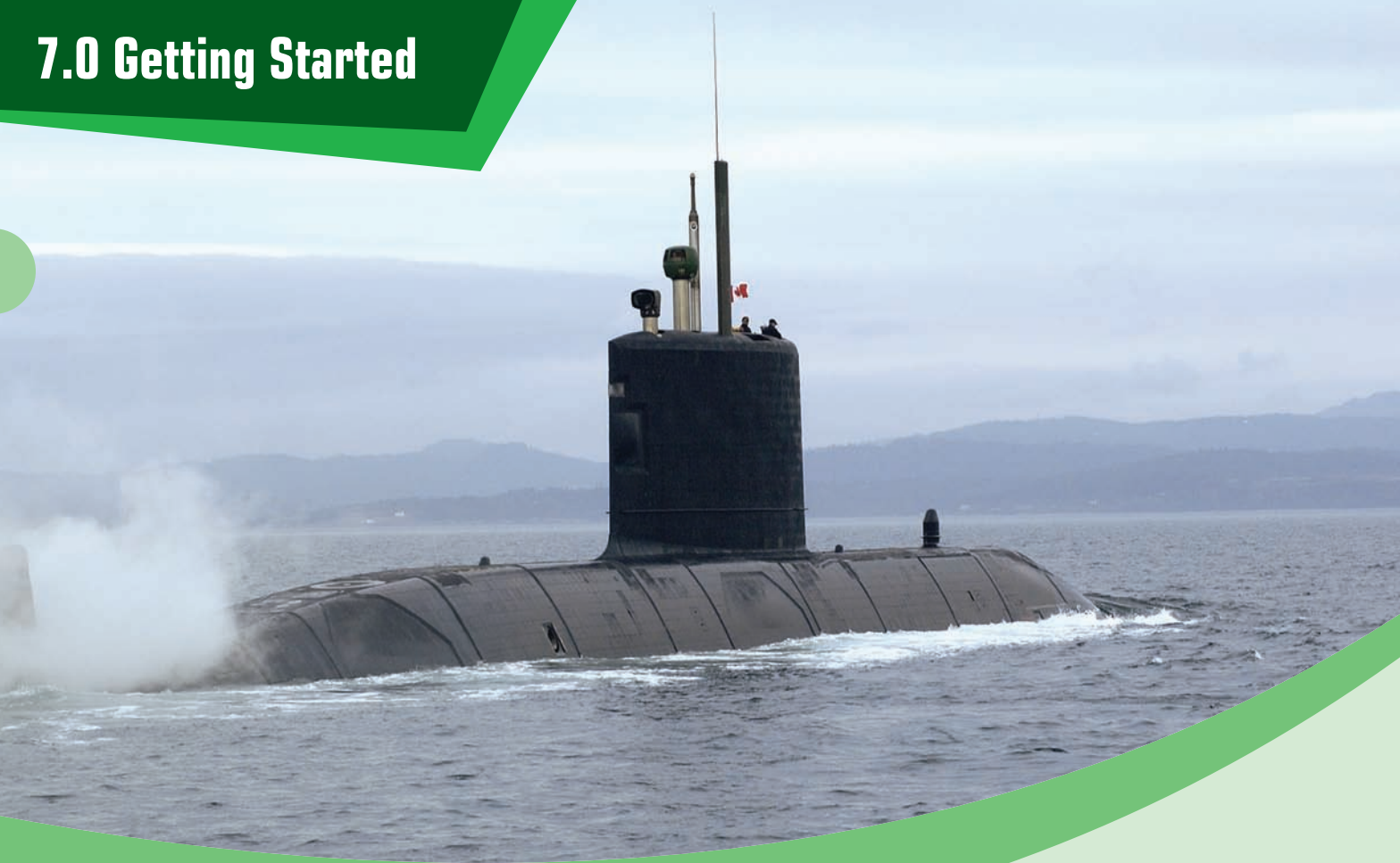
Figure 7.1 HMCS Victoria is one of Canada's four diesel-electric patrol submarines. Each submarine of its class is over 70 m long and can dive to a depth of more than 200 m.
