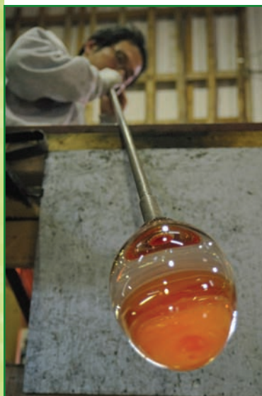
Figure 7.15 Blowing molten glass with a blowpipe
