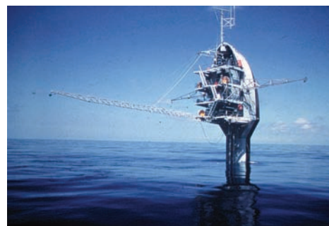
Figure 8.16 FLIP is a research platform that floats out to sea. The platform becomes vertical when water is pumped into its tanks.
