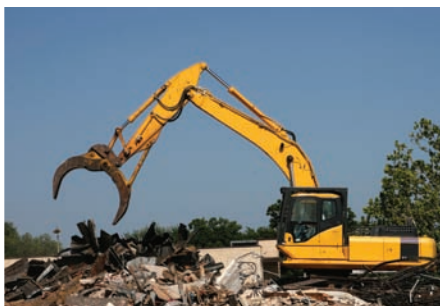
Figure 9.7(a) Hydraulic systems are used to move materials, such as rock, soil, and scrap metal.
