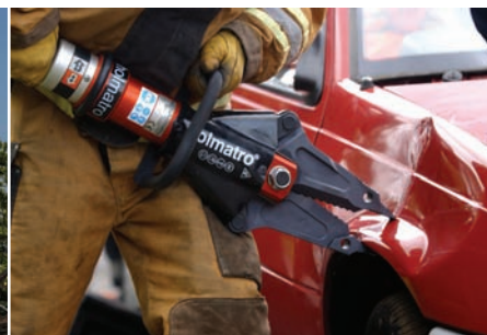
Figure 9.7(b) Rescue workers use hydraulic systems in the Jaws of Life ® to free people trapped in vehicles.
