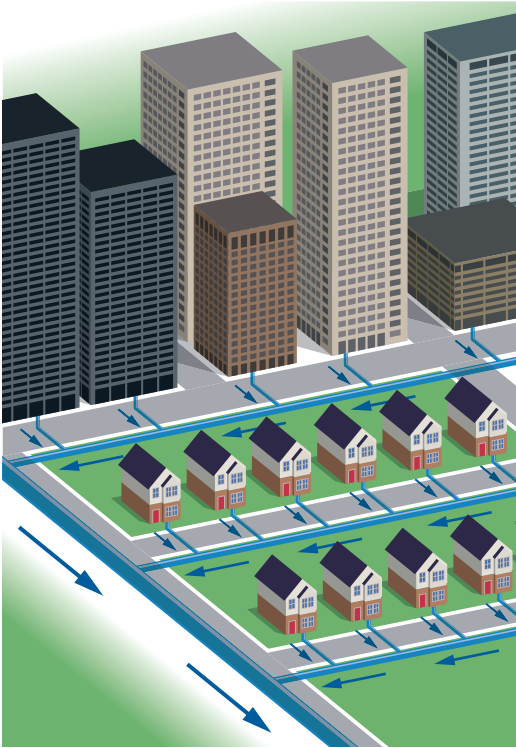
Figure 11.15 All of the waste water in your home goes into an underground collection system of pipes.
